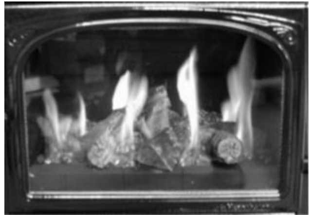
Figure 21 – Typical Burner Flame Appearance
